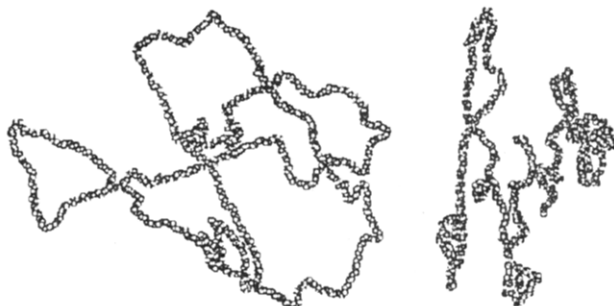
Figure 2. Two views of the coil conformation of the parent chain in a film formed with a poly(1,4- trans -butadiene) chain of 180 repeat units after a molecular dynamics simulation of 1500 ps at 300 K. Left: XY projection (X horizontal, Y vertical). Right: YZ projection (Z, horizontal, Y vertical).
